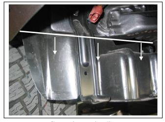
Figure 5: Cut under steel radiator support
