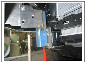
Figure 4 – lower bolt through under body guard
